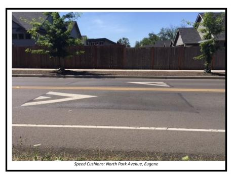
speed bumps which are typically found in parking lots and jar motorists regardless of speed, speed humps and speed cushions have a more gradual slope, forcing motorists to slow down. To reduce impediments to emergency vehicles, speed cushions have wheel cutouts to allow large vehicles to pass unaffected, while reducing passenger vehicle speeds. The following procedures are intended to ensure neighborhood support and appropriate use of speed cushions on a road prior to installation.
